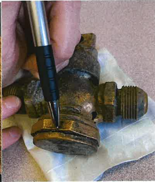
Corroded cc base
